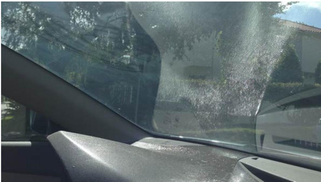
16. As seen above, drivers' views are obstructed by the glare from melting dashboards. The dashboards' shiny surfaces create a reflection on the windshield making it difficult for drivers to see.
