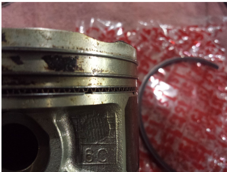
FB20 Piston with Worn Oil Control Ring
