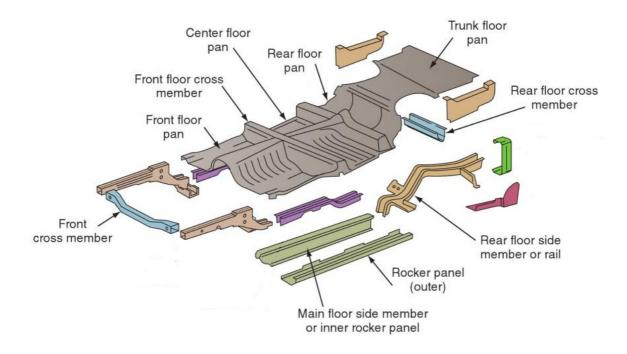
31. The front floor pan is a single piece of metal that spans the front driver and passenger compartments forming the floor of the vehicle for the front passenger and driver. Normally the floor pan is covered in carpet. Floor pans are intended to last the life of the vehicle and are not a "wear component" that owners or service technicians expect to repair or replace during the vehicle's anticipated useful life. A floor pan schematic appears below:
