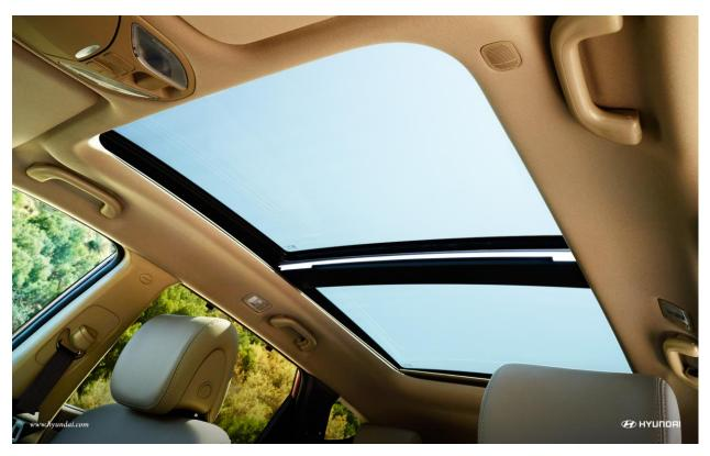
18. Hyundai makes its panoramic sunroofs out of tempered glass, also known as toughened glass. In the automotive industry, tempered or toughened glass is generally made by shaping and cutting a piece of annealed glass that is then heated and rapidly cooled. This tempering process creates an outer layer of compression that is shrinkwrapped around the middle of the glass, which is constantly pressing outwards, making
