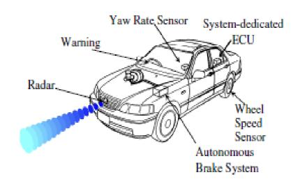
18. The Honda Sensing system in Class Vehicles employs a millimeter wave radar unit (on the front of the vehicle near the bumper) as well as a camera (located near the rearview mirror). For CMBS purposes, the radar and camera scan approximately 100 meters ahead of Class Vehicles searching for potential obstacles that could cause a collision. If an obstacle is detected, the CMBS will alert the driver and potentially apply light or strong brakes automatically.
