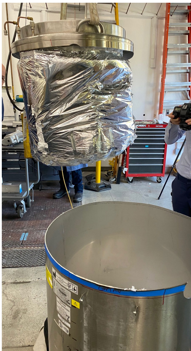
28 Tank 4's inner vessel suspended after removal from outer vessel (vacuum space was in between)
