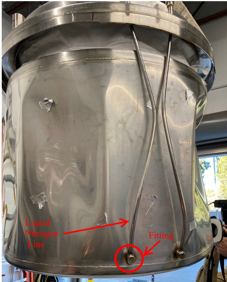
10 11 12 13 14 15 16 17 18 19 20 21 22 23 24 25 26 27 28 Liquid nitrogen tube feeds into Tank 4's inner vessel
