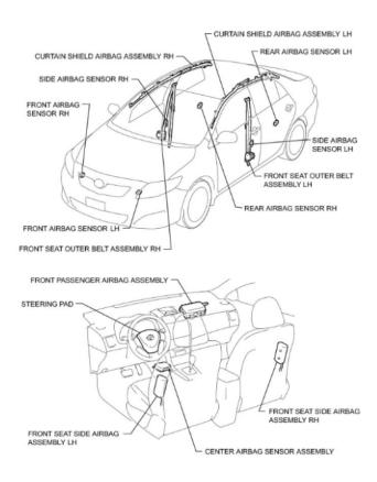
35. The ACU contains an electronic component—an application specific integrated circuit ("ASIC")—which monitors signals from other crash sensors located in the Class Vehicles. If the ASIC fails, the ACU will not operate properly and airbags and other supplemental restraints will not deploy when needed. *See* NHTSA ODI Resume, Investigation EA 19-001.
